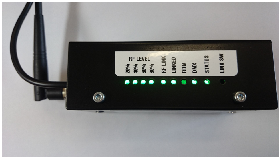
Wireless module in receiver mode with full signal.
